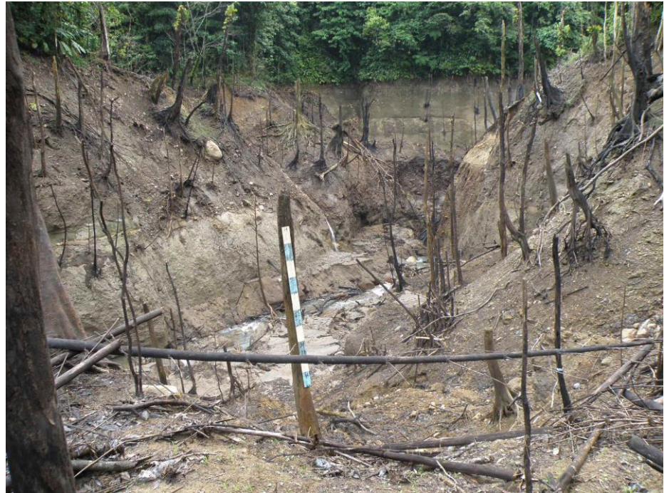
Some of the staff gauges remained completely submerged for several years before Matthieu Lake emptied following collapse of landslide plug
